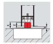
Calculating the necessary length of spindle extension: Extension = X - Floor clearance (normally 8 mm)
